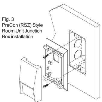
Mounting hardware is provided for both junction box and drywall installation (junction box installation shown) for the Delta Style and PreCon Style room units. Mounting hardware is provided for only the drywall installation of the Powers style room unit. Junction Box installation of the Powers style room unit will require an adaptor plate. Order Part Number BA/ADP-525-7-Color Code.
